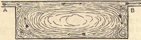
Fig. 113.—Ex.—Whirl Flattened by Restraint.
